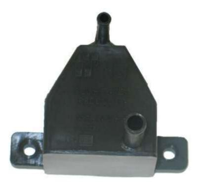
To test the valve, blow air through either port. The valve is open and air should flow freely through both ports when in its normal position as mounted on the tank. When positioned up-side-down as shown, the valve should close and permit no airflow through the
