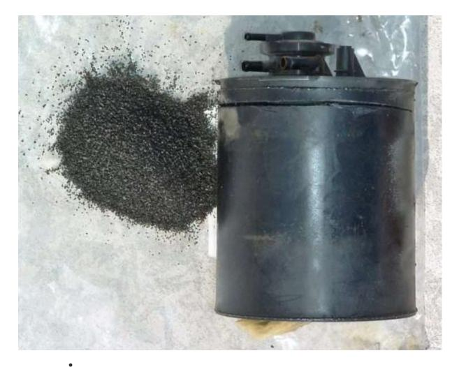
EVAP Filter. A virtually unknown filter is under the lower cover and cleans the air going into early EVAP canisters. The factory service manual says to change the filter at least every 24 months or 24,000 miles. I've never seen or heard of one being replaced but they are available.
