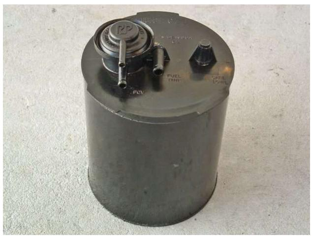
Carbon. The carbon inside the EVAP system's canister stays effective for many years. With early EVAP canisters, the carbon can be removed and replaced. A common source of activated carbon is aquarium supply stores for their filters.
